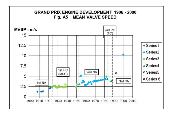
Interference-fitting double coil valve springs and better-quality vacuum-refined, shot-peened wire then raised MVSP gradually for the universal Coil-spring Valve Return Systems (CVRS). Inlet *and* exhaust valves in Ti-Alloy for NA engines helped from 1989 by reducing their mass, stems also being drilled for the same reason. These improvements pushed MVSP up to 4 m/s.
