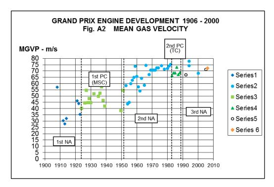
Note 34 discusses in detail the optimum value of MGVP when the highest product of (EV x EC) is the target. In particular it explains that PC engines can operate best with a lower value than NA because the mixture is heated and "mashed" in the compressor.
