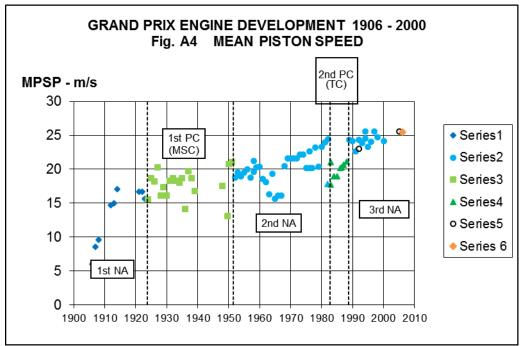
Although Al-alloys for the piston became available generally in WW1 their post-war use only just preceded the application of Pressure-Charging, which placed greater pressures and temperatures on that part, so that the average MPSP in the 1PC era did not rise significantly.
