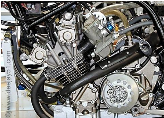
Fig. 17 SO18 1965.5 Honda RC149 Transverse 5 a/c 35.5 mm/25.1 = 1.414 124 cc 32.7 HP @ 20,000 RPM
