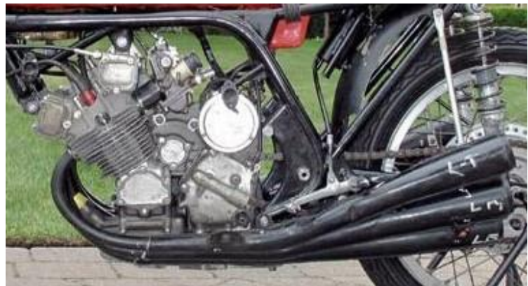
Fig. 18 1966.5 Honda RC174 Transverse IL6a/c 41 mm/37.5 = 1.093 297 cc 68 HP @ 15,500 RPM
