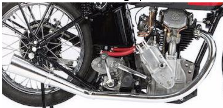
Fig. 5 PEP 206 1939 Excelsior Manxman 350 Vertical 1 a/c 75 \text{ mm}/79 = 0.949 249 cc 22.5 HP @ 6,000 RPM
