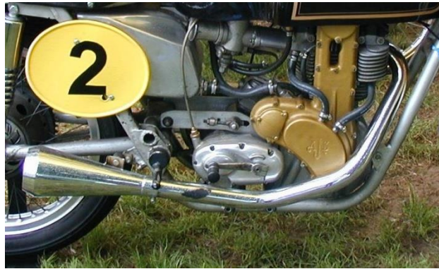
Fig. 16 SO15 1962 AJS 7R Vertical 1 a/c 75.5 mm/78 = 0.968 349 cc 42 HP @ 7,800 RPM
