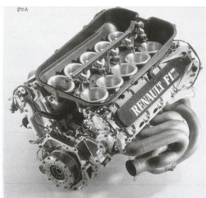
Fig. 80A 1996 Renault RS8 67V10 *92/45.1 = 2.04 2,998 cc* DASO 1017 It is likely that the all-new RS9 had already been designed when the Renault management in June 1996 decided to leave F1 at the end of 1997. Otherwise they would hardly have gone to such expense.
