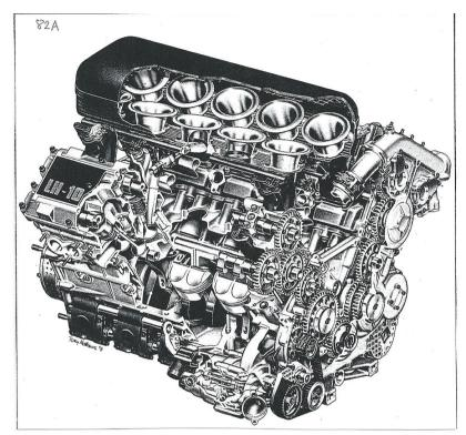
Fig. 82B The camshaft gear drive of the FO110G was at the front, as in all Ilmor F1 Engines, where their V8 Indy engine had it at the rear.
