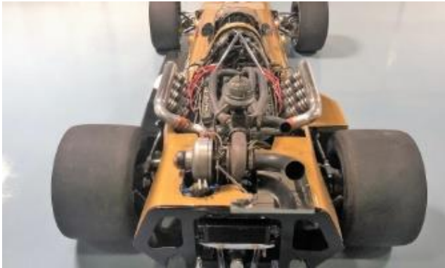
TurboCharged Ford 4-Cam 1969 90V8 95 mm/46.5 = 2.04 2637 cc
